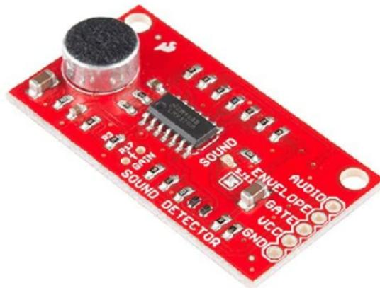
Figure 7-3 SparkFun Sound Detector
