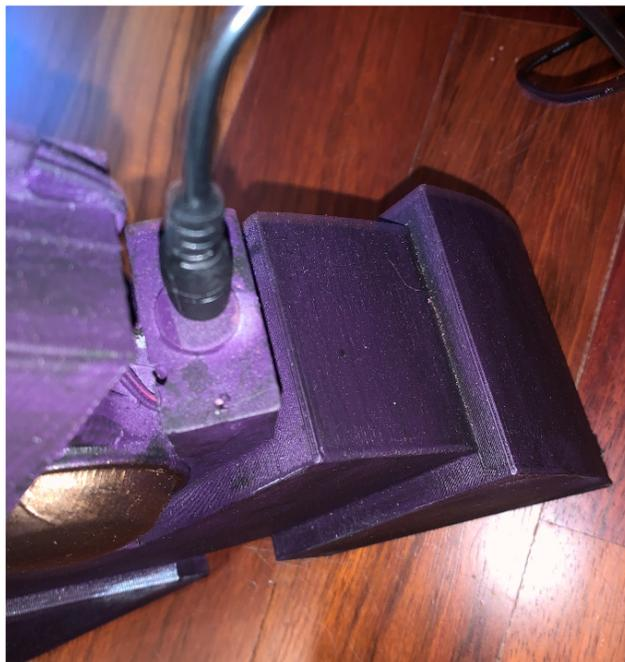
Figure 3-2 DC Barrel Jack Holder Installed
